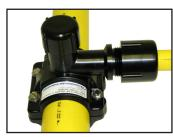
Tighten the compression nut until it shoulders against the outlet. Do not overtighten. **CAUTION:** To prevent inadvertent pull-out of the P.E. tubing during the assembly process, complete step 11 immediately after step 10, without delay and ensure work is not being performed on the free end of the P.E. tubing.
