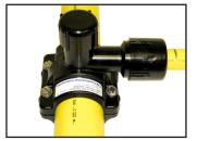
**12** Line marked for stab depth should be no more than 3/4" from face of compression nut.
